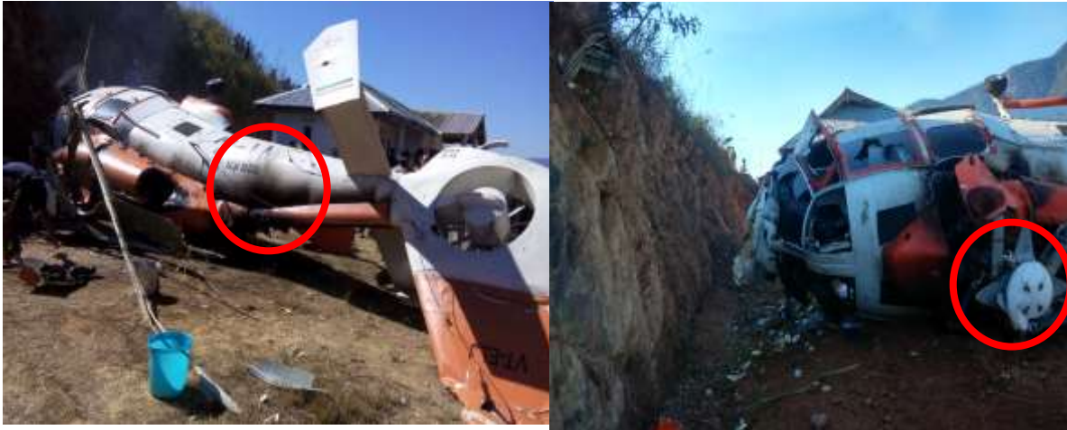
Fire marks on front tail boom area
